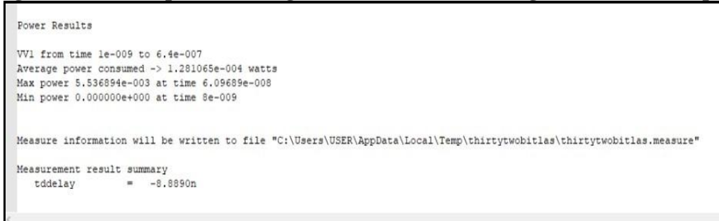
Figure No.13: Power and Delay analysis for the proposed Sorting network with 32-bit weighted bitstream input
